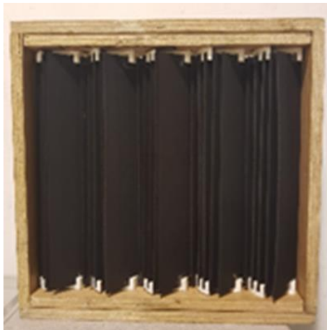
Biochar fins can be arranged and fitted into air duct
